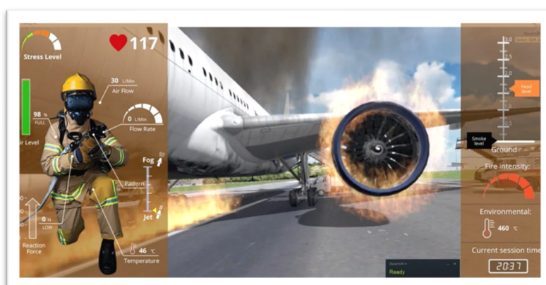
Figure 25: Screenshot of the trainer's view. The trainee's vitals on the left, view from inside the program in the middle, and general environmental statistics on the right [24].
