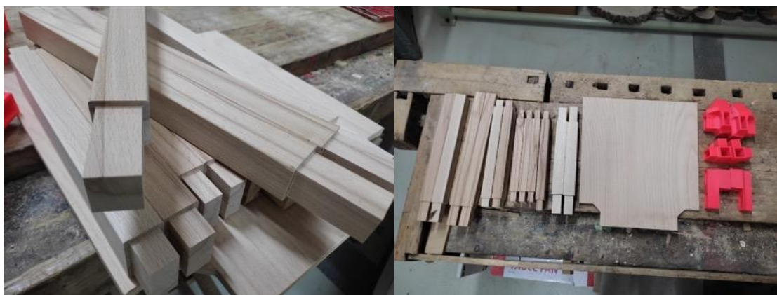
Figure 120: Chair wooden parts preparation.
