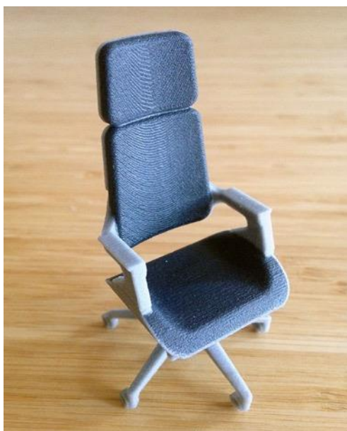
Figure 23: HOSU office solutions prototype of a 7 cm highchair [26].
