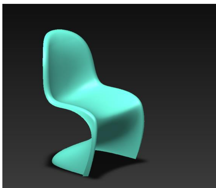
Figure 92. Joined, filleted, and mirrored faces into one final surface.
