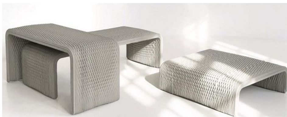
Figure 21: Printed concrete benches with a complex weave pattern, by the startup XtreeE in collaboration with the design studio Studio 7.5 [24].
