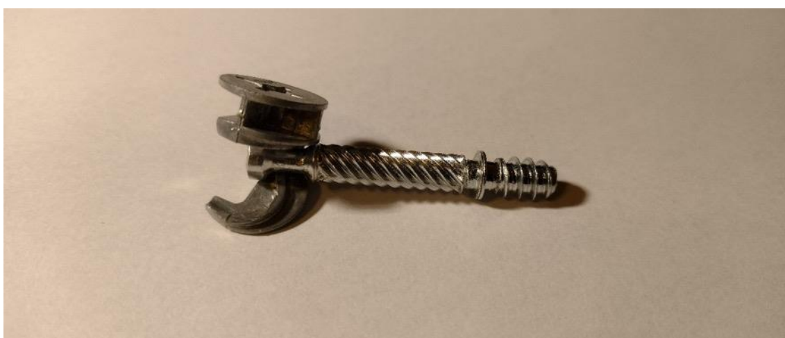
Figure 40. Connector flange with broken off (almost) piece.
