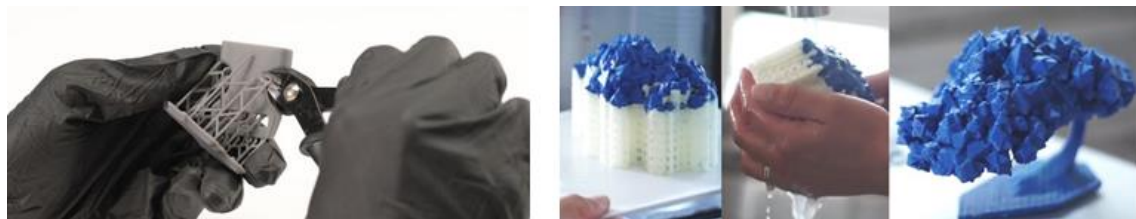
Figure 11: Mechanical process and bath for removing the support structures [13] [14].
