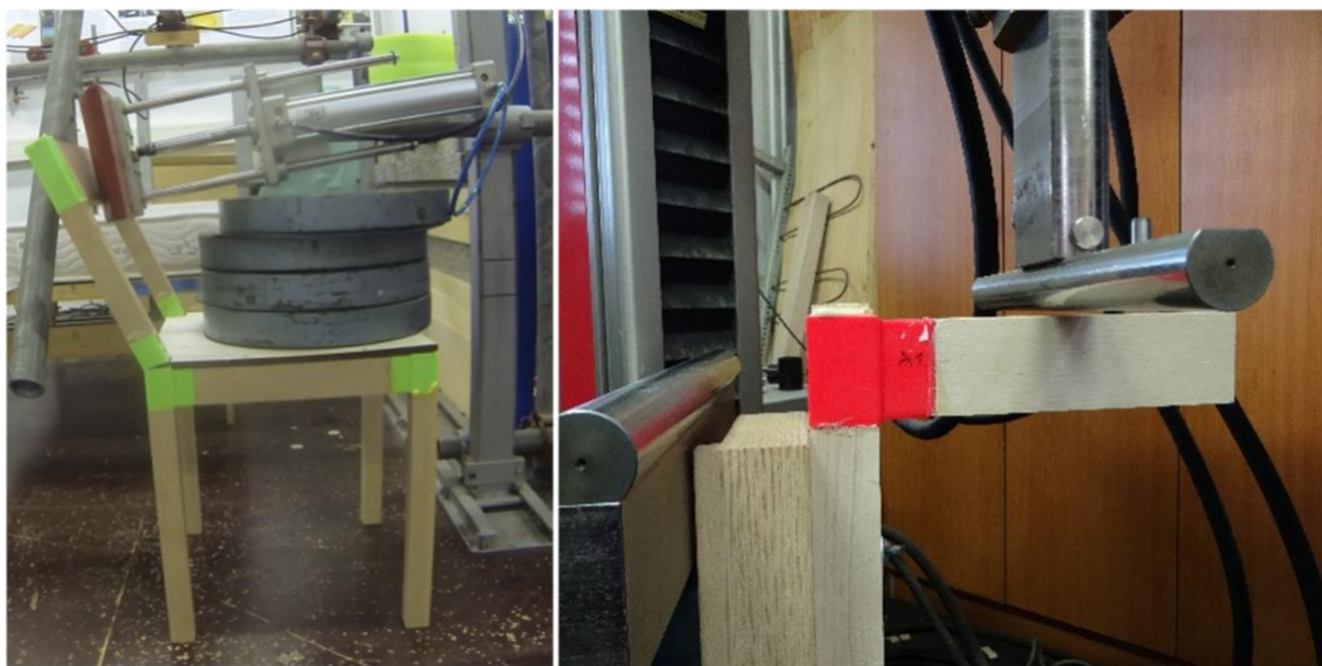
Figure 124: chair testing according to standard EN 1729- left; connector testing – right.
