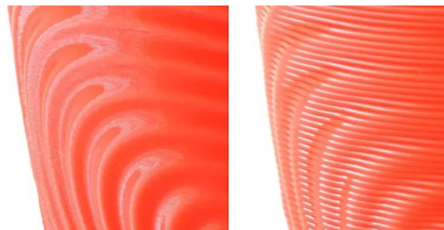
Figure 9: 0,2mm Layer Height (Left) vs 0,9mm Layer Height (Right) [10]
