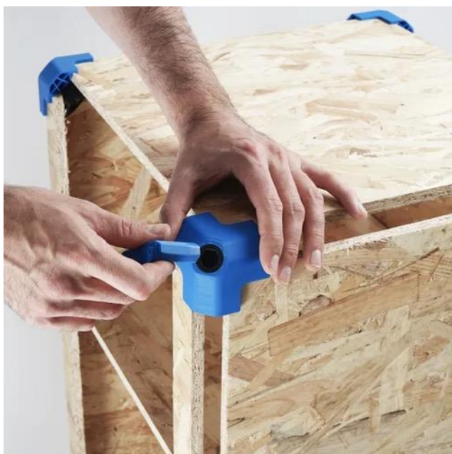
Figure 25: Connecting parts for three-dimensional assemblies created by Jean-Charles Roderger's Alternative Design Lab [28].
