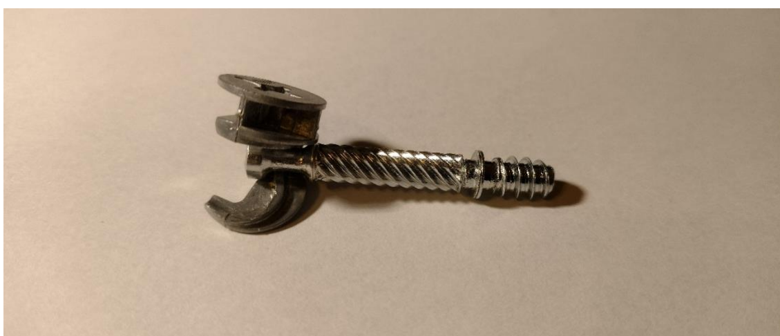
Figure 7. Connector flange with broken off (almost) piece.
