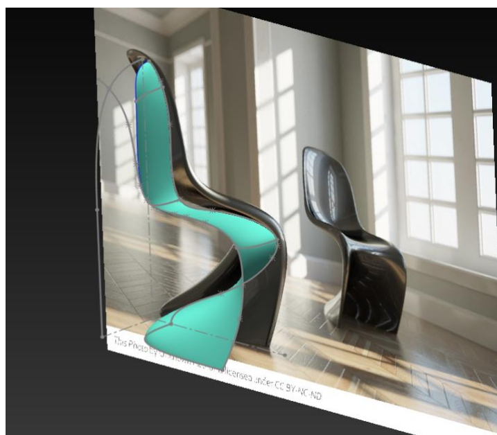
Figure 49. Chair seat formed from projected and bottom curves.
