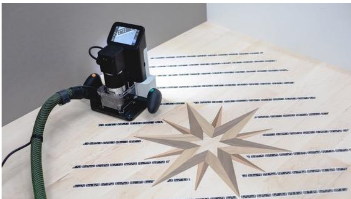
Figure 28: Medallion Flooring Inlay with Shaper Origin.
